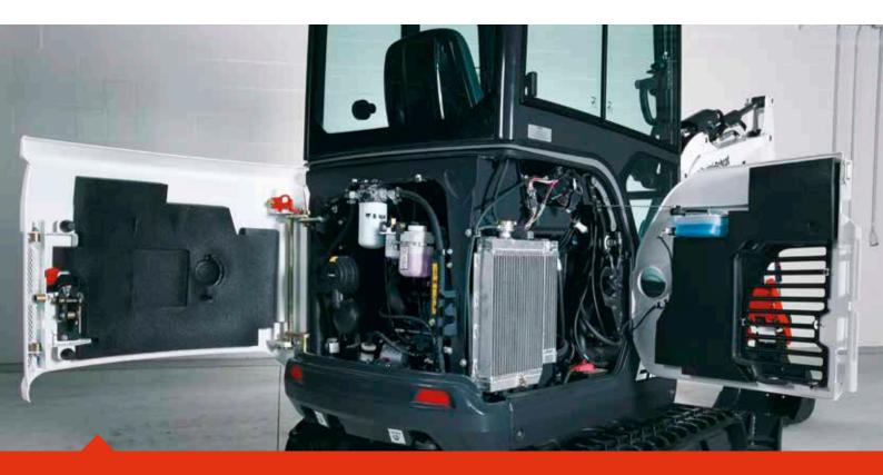
Side-by-side coolers for easy cleaning. Diagnostics are easy thanks to display error codes on control panel and service tool connection. With all openable covers the E17, E17z, E19 and E20z provide best-in-class access in their categories to all daily maintenance components and service points.
