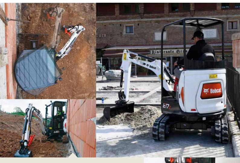
The Zero House Swing (ZHS) concept enhances Zero Tail Swing (ZTS) functionality by further protecting the front upper structure corners turning within the swing circle. ZHS functionality provides 320° of free rotation while working close to any object.
