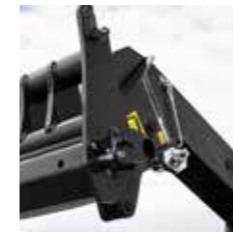
Hydraulic attachment locking using a dedicated auxiliary line
