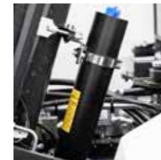
Boom suspension (Nitrogen accumulator)
