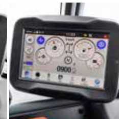
7" touch display with built-in Bluetooth radio, microphone, loudspeakers, phone page and Job Manager
