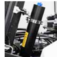
Boom suspension (Nitrogen accumulator)
