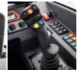
Smart joystick with Boom float and bucket shaking
