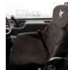
Air suspended seat with headrest
